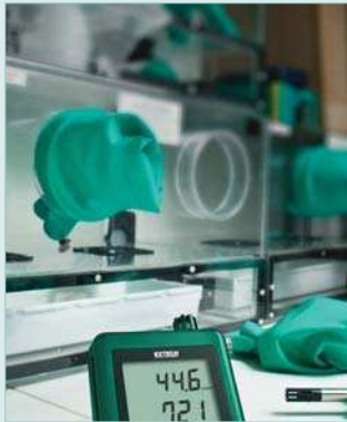
Monitor and record temperature and humidity values in the calibration rooms, office, clean rooms, and storage facilities
